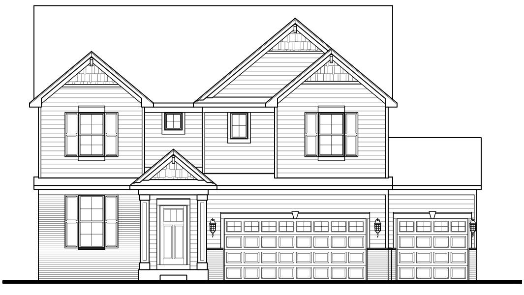
Front Elevation E Scale : 3/16"=1'-0"
